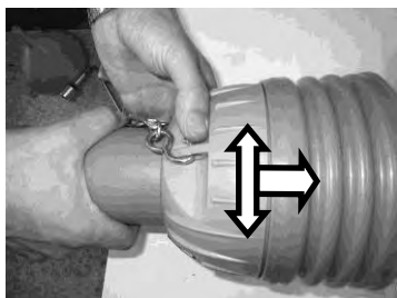
Turn the casing to phase it
