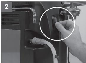
**Step 2.** Check the “Battery Indicator” that sufficient power is available, if not connect to the AC or DC adaptor.
