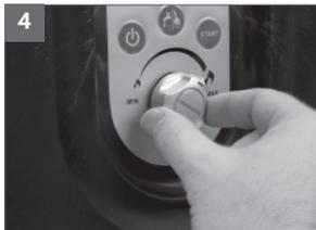
**Step 6.** The water temperature can be adjusted by moving the flow valve between “Min & Max” as this will slow or increase the water flow resulting in an increase or decrease in the outlet temperature.
