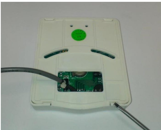
Figure 7-Pop off the rear cover of the interface using a flat head screwdriver or similar
