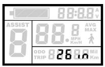
Press **MODE** to confirm the wheel size and enter into the LCD backlight brightness setting. The default value of the wheel size is 26 inch.
