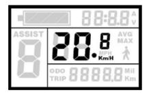
Hold **UP** and the display will show the MAX speed during this ride. Hold **UP** again and the display will show the AVG speed during this ride. Hold **UP** again and the display will turn to the current speed display.
