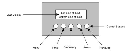
Operation of the instrument is controlled by push buttons. These are labeled as in the diagram above.
