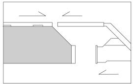
**2.** Align debris bag. Material sleeve will slip up over the extension tube and handle.
