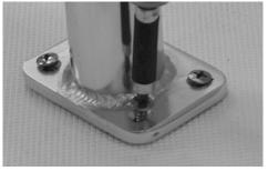
Remove the Frame Canopy to Complete the Standoff Installation: Once the bases are partially screwed into the deck of the boat remove the Four (4) upper leg clamps and the Canopy Frame as shown below. The reason for this is moving the clamps on the top section frame during alignment will scratch the finish of the aluminum. This also allows the legs to be more accurately aligned vertically.
