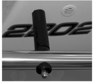
Complete the first standoff installation <u>using Loctite</u> tightening both the Acorn Nut and Backing Plate Nut.
