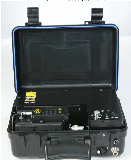
(fig. 2-3) – PHT Case (opened with CMT installed)
