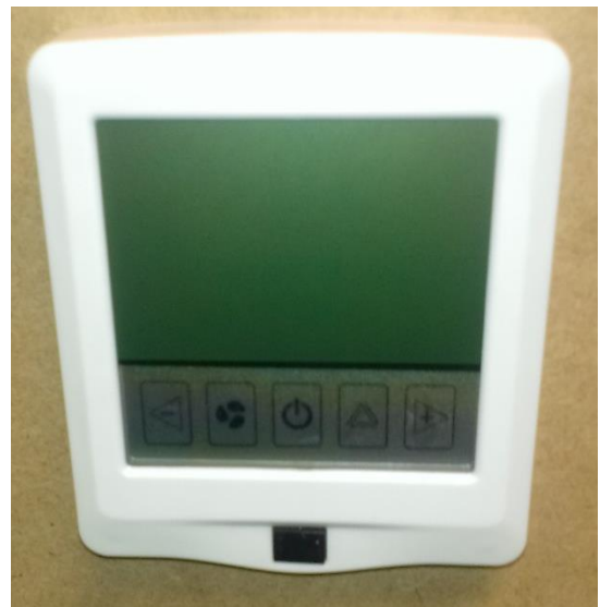
Figure 9-Replace the front cover of the interface
