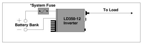
\* A system fuse (of at least 40 Amps) should be placed before the battery. An HRC motor start type is recommended. (See your system designer for details).
