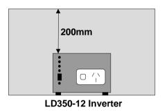
Please leave a clearance of 200mm on all sides and top of the Inverter. The LD350-12 must be installed in a dry, cool, dust-free environment. It is recommended that the inverter be placed as far from any radio receivers as possible.
