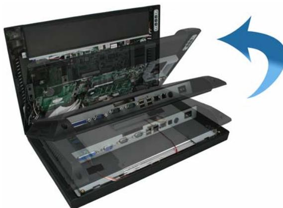
3. Separate the back panel from the front panel by lifting up and lay it down carefully.
