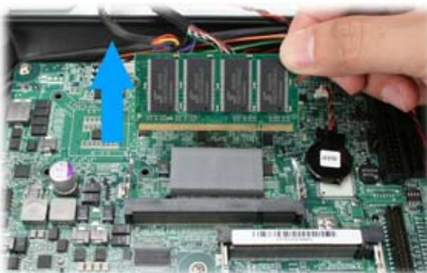
5. Align and insert the new RAM in the slot and push both ends of the RAM down until the ejectors snap into place.
