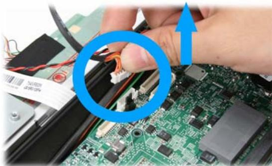
2. Unplug the power switch cable from the mainboard as shown below.
