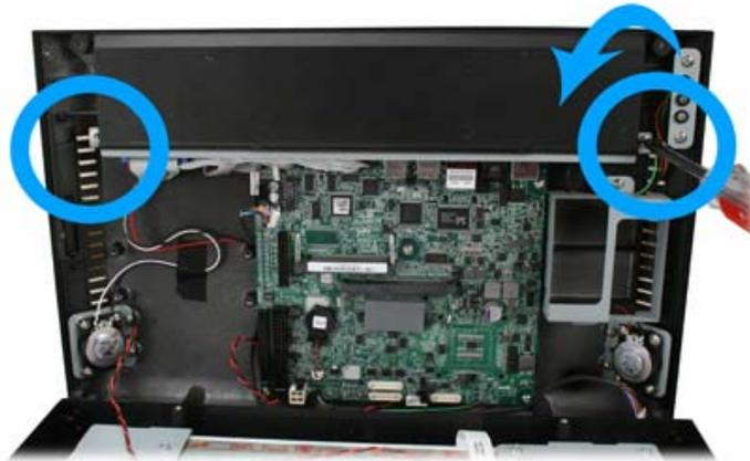
5. Loosen the five screws by #0 Phillips screwdriver as shown below.
