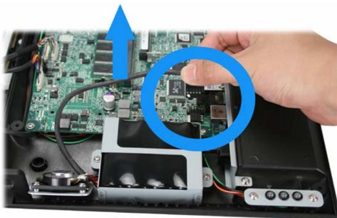
2. Loosen the two screws by **#1 Phillips screwdriver** as shown below and remove the battery.
