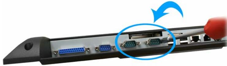
4. Remove the two screws by #1 Phillips screwdriver as shown below.
