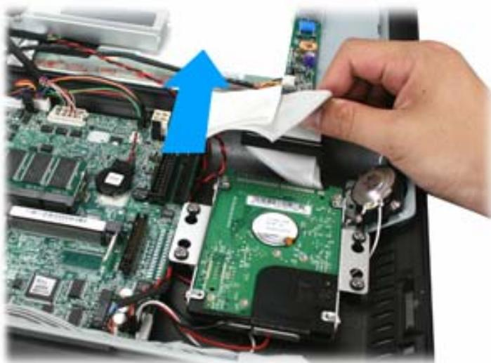
3. Loosen the four screws by #1 Phillips screwdriver as shown below and remove the HDD assembly from the device.
