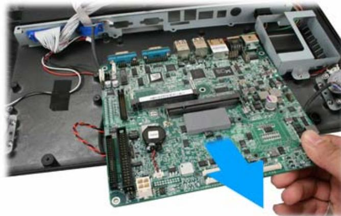
7. Remove the I/O panel from the device as shown below.
