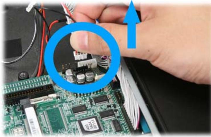
5. Unplug the speaker cable from the mainboard as shown below.
