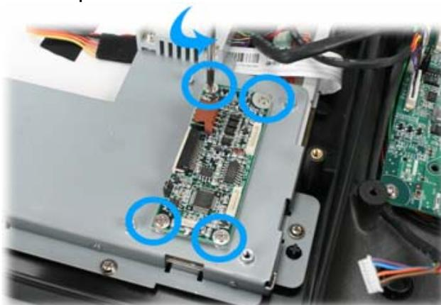
2. Install the new touch panel control board in the reverse procedure.
