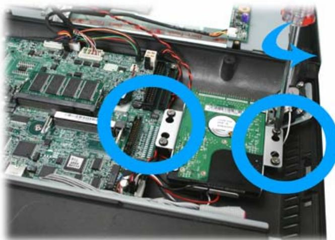
4. Loosen the four screws fixing the HDD and remove the HDD from the bracket as shown below.
