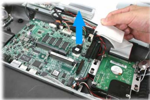
2. Unplug another connector of the IDE cable from the HDD.
