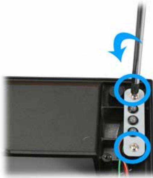
12. Loosen the screws fixing the speakers and you can remove it from the device.
