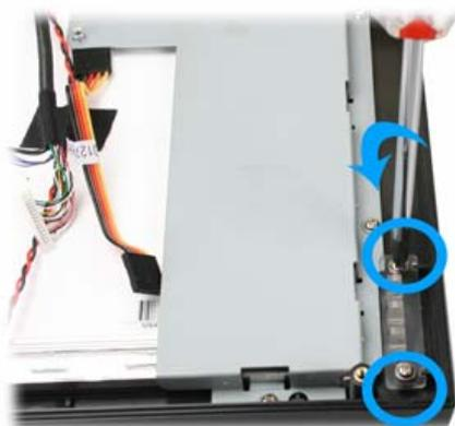
2. Loosen the eight screws in blue circle as shown below by #1 Phillips screwdriver.
