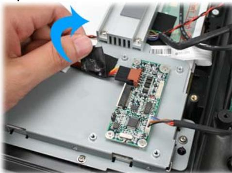
2. Disconnect two connectors from the touch panel control board as shown below.
