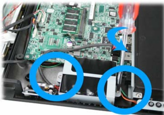
3. Remove the battery and the battery bracket as shown below.
