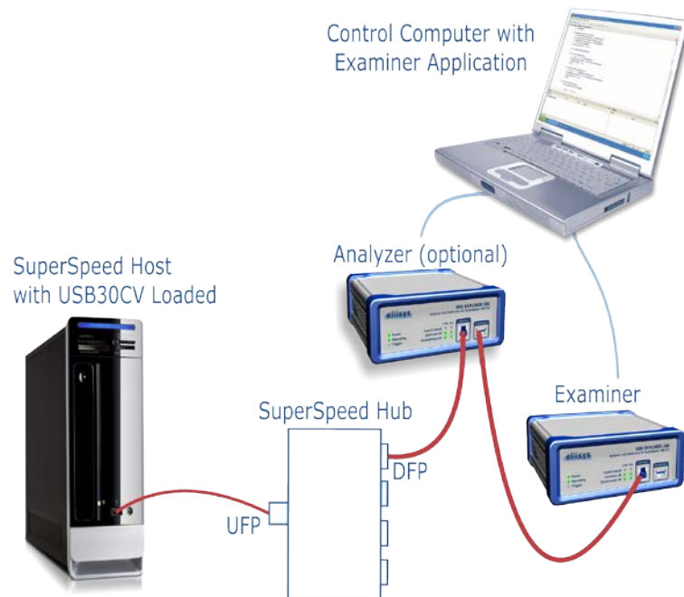
Figure 3-4 Examiner Setup for Testing Hub Downstream-Facing Port
