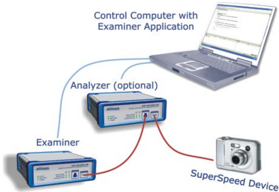
Figure 3-2 Examiner Setup for Device (or hub upstream port)
