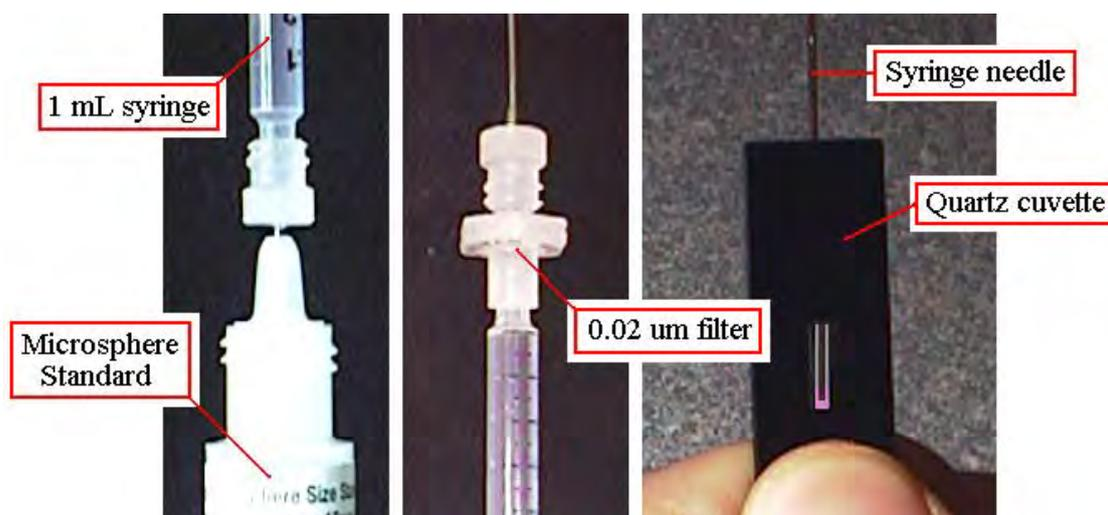
The cell is now ready to be loaded into the DynaPro. Note that there is an opaque or frosted side on the cell. **The frosted side of the cell must be positioned to the left side of the optics block.** After seating the cell in the DynaPro optics block, close the lid to de-activate the laser power safety (kill) switch.
