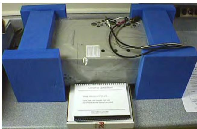
Inspect the instruments for visual shipping damage and report obvious trouble to our technical support department. Then place the Host unit and the MicroSampler close to the computer which will be used to operate the DynaPro.
