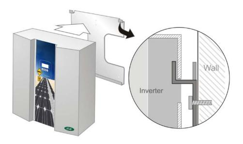
Step3. Make sure that the GT is positioned securely on the bracket.
