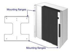
If you do not want to use the supplied wall mounting bracket as a template, observe the dimensions shown in the drawing above. The procedure for mounting the inverter using the wall mounting bracket is described on the following pages.
