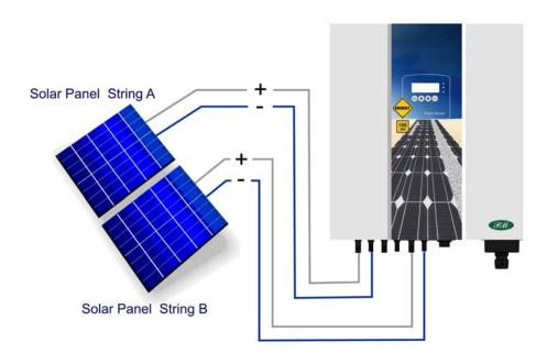
Fig. 5 DC Connections for a Two-String PV Array
