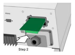
Put the communication card into the slot
