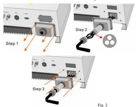
Step 4. Insert utility wires through cable gland. Connect wires according to polarities indicated on terminal block.
