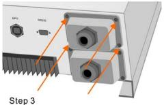
Screw back the side & top cover and complete the installation
