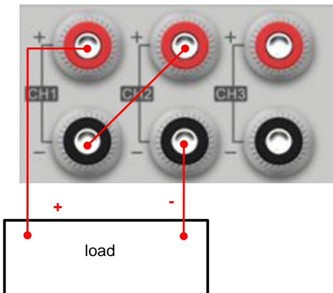
Figure 3-5 Wiring diagram for Series mode
