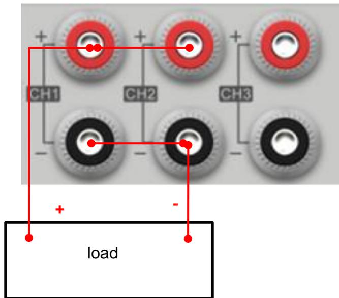
Figure 3-7 Wiring diagram for Parallel mode
