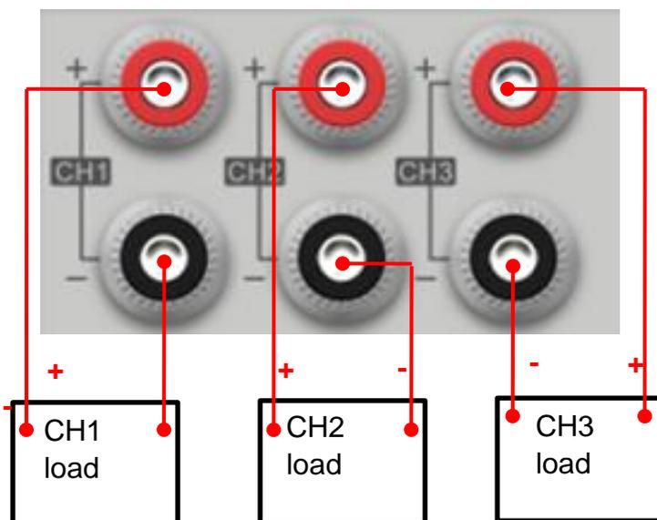
Figure 3-3 Connection diagram for Off states
