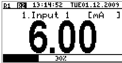
Fig. 6.22. Screen with relay 1 open and relay 2 closed.
