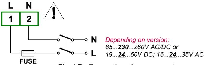
Fig. 4.7. Connection of power supply
