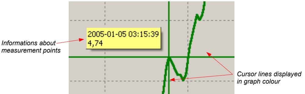
Fig. 3.9. Graph with special tracking cursor
