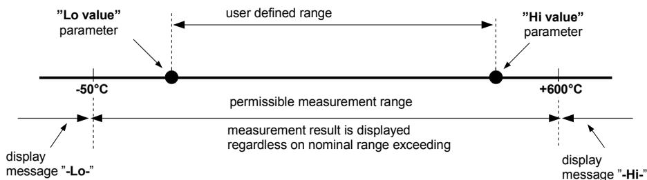
Fig. 6.1. Definition of measurement ranges
