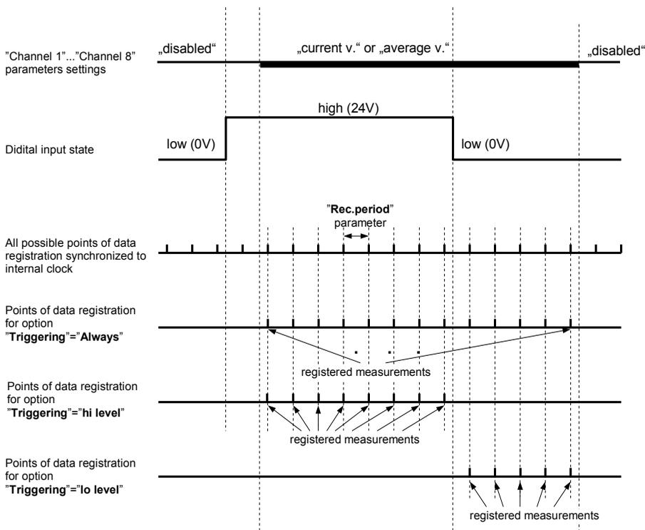
Fig. 7.18. Recording points depending on **“Triggering”** parameter value.
