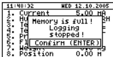
Fig. 7.15. Warning in "until full" recording mode
