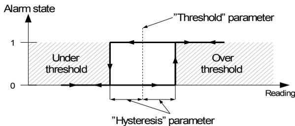
Fig. 6.23. **"Over threshold"** mode diagram. 0 means alarm not present, 1 alarm present
