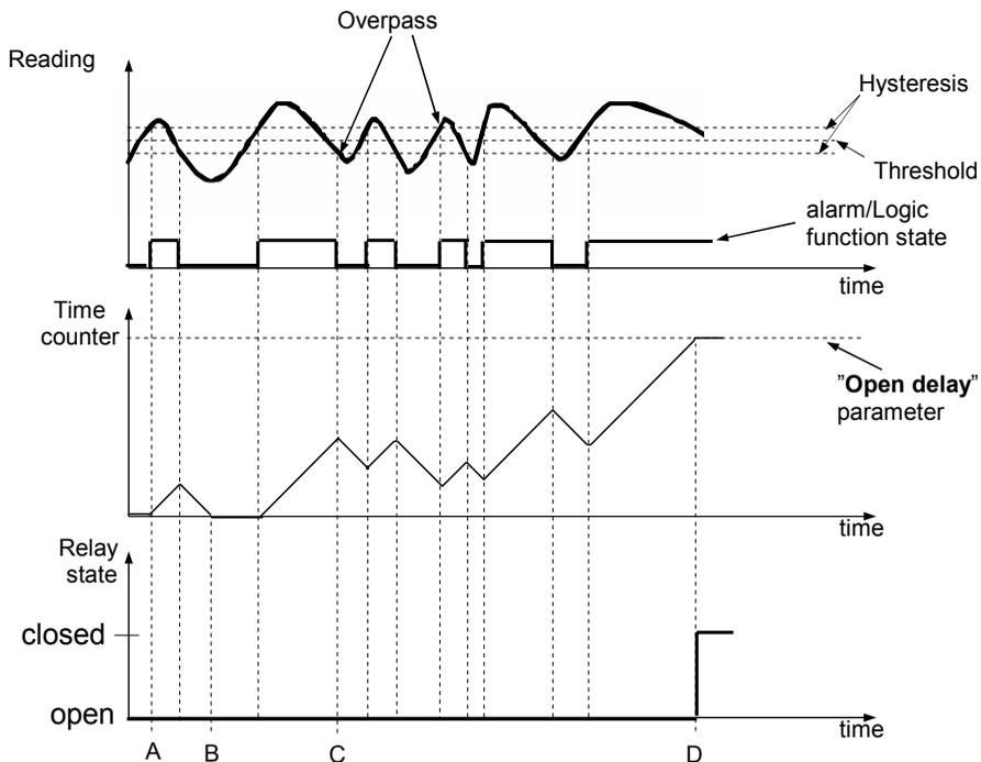
Fig. 6.27. Working output controlled by single channel alarm with large reading oscillations. Alarm mode - "over threshold", "Open hold time" and "Closed hold time" equals 0, "Open delay" and "Close delay" greater 0.
