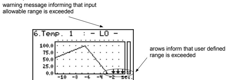
Fig. 6.16. Exceeding lower limit of the allowable measurement range
