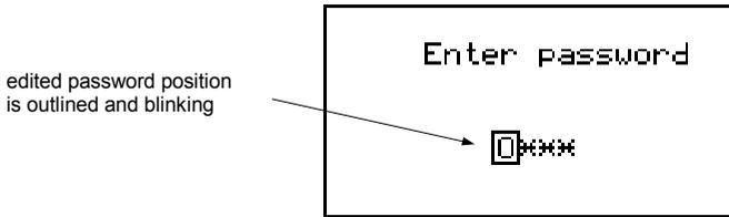
Fig. 7.2. Password requested when accessing unit's main menu.
