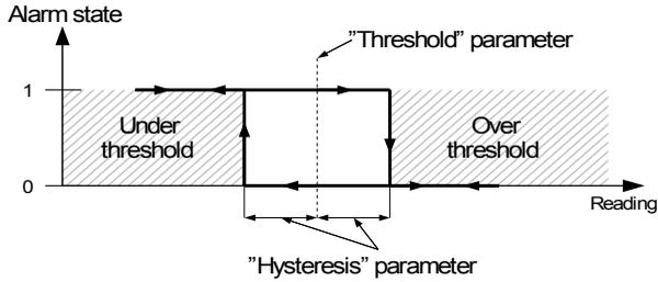
Fig. 6.24. "Under threshold" mode diagram. 0 means alarm not present, 1 alarm present
