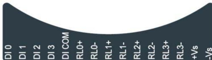
Figure 2.24 WISE-4060 Pin Assignment
