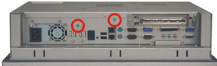
Figure 4-6: Elevated Platform Retention Screws (Bottom Panel)
