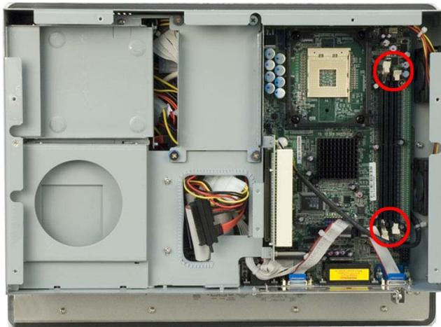
**Figure 4-8: DIMM Socket Clip Locations**
