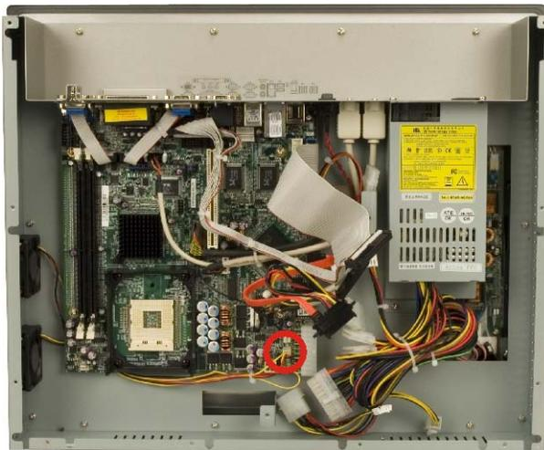
Figure 4-13: System Cooling Fans Motherboard Connector
