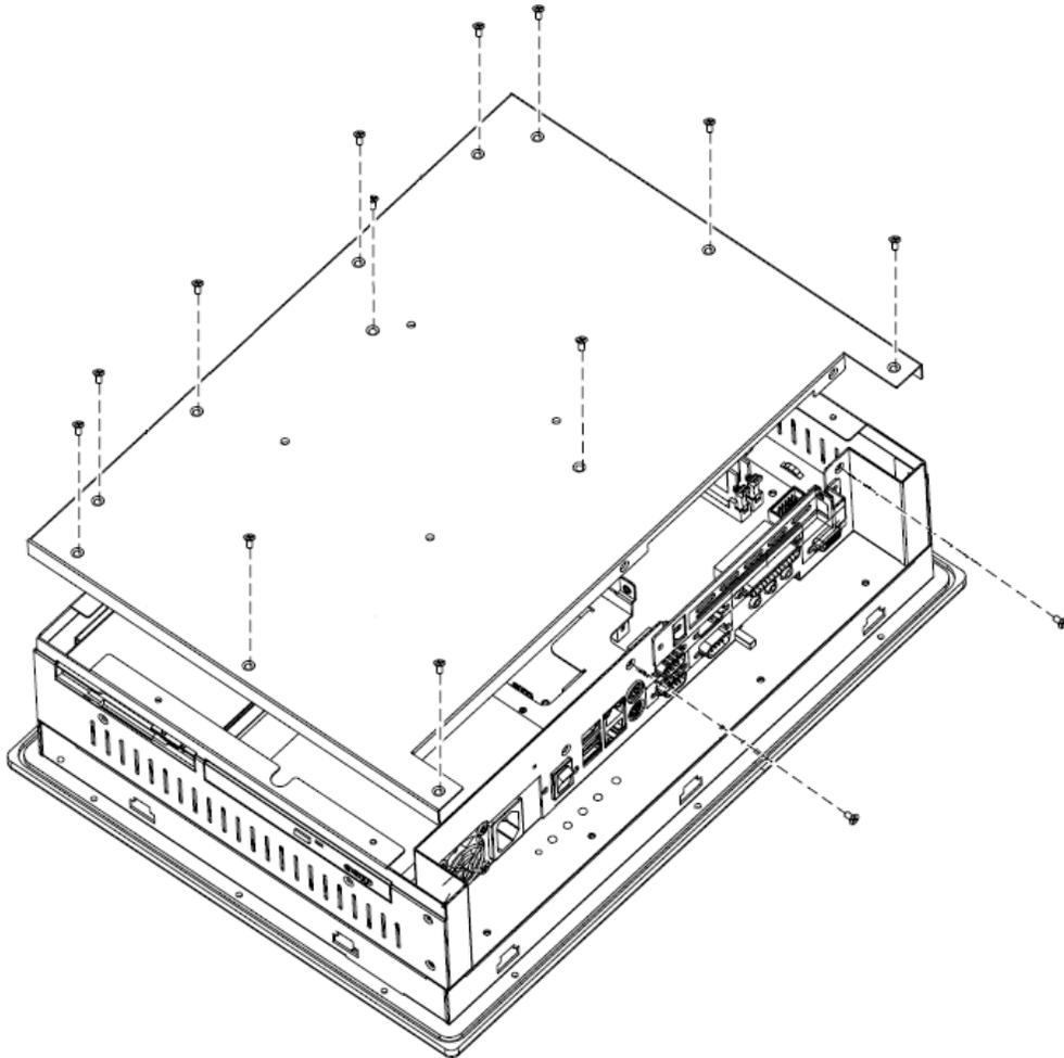
Figure 3-1: Back Cover Retention Screws
