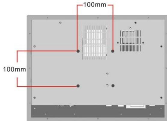
**Figure 3-18: Arm Mount Retention Screw Holes**
