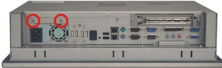
**Figure 4-2: CD Drive Retention Screws**
