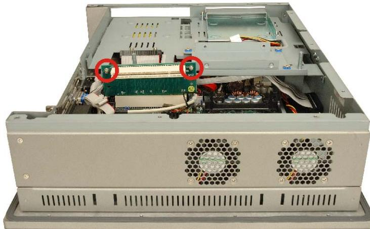
Figure 4-7: Elevated Platform Retention Screws (PCI Riser Card)
