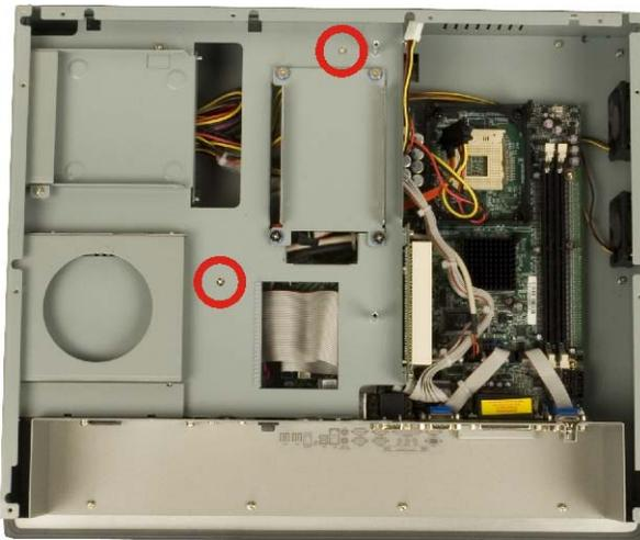
**Figure 4-3: Internal Elevated Platform Retention Screws**
