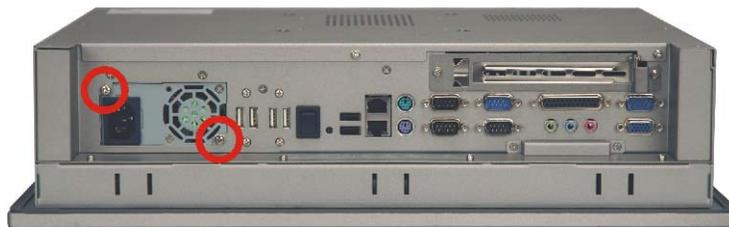
**Figure 4-10: PSU Bottom Panel Retention Screws**
