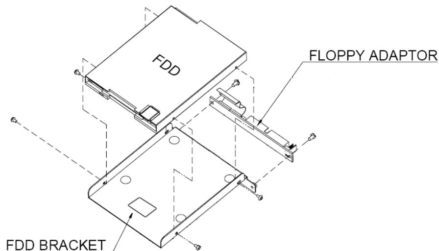
**Figure 3-4: FDD Adapter and FDD Bracket Installation**
