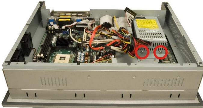
Figure 4-12: PSU Bracket Retention Screws
