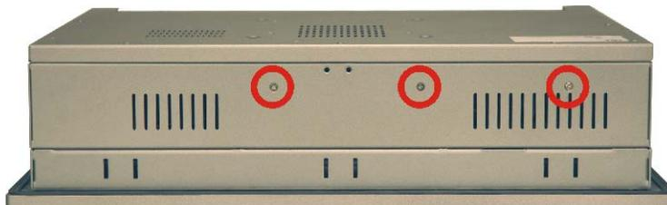
**Figure 4-4: Elevated Platform Retention Screws (Top Panel)**
