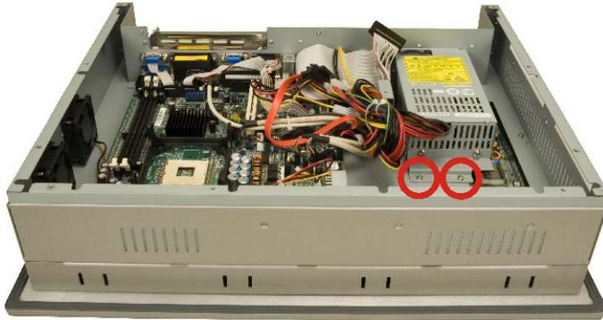
Figure 4-11: PSU Bracket to Chassis Retention Screws
