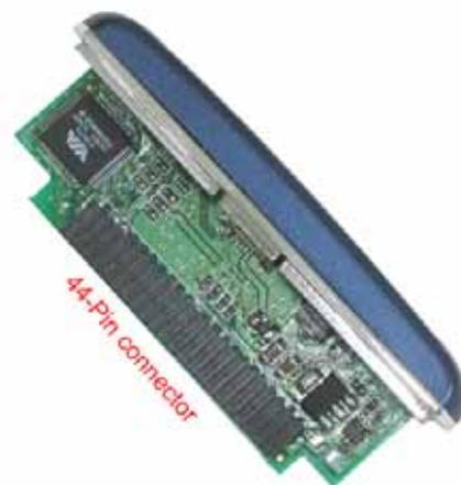
3. Connect 2.5" HDD into the 44-Pin connector on circuit Board.
