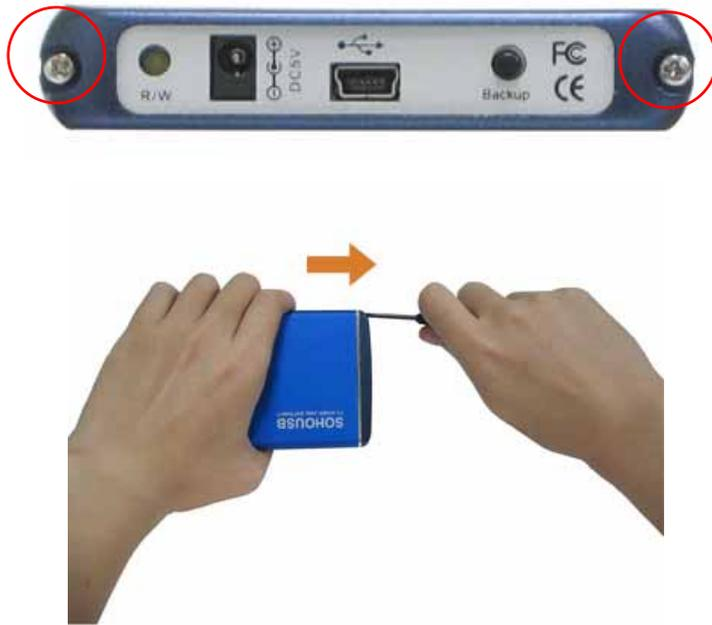
2. Pull out the plastic cap with circuit board.
