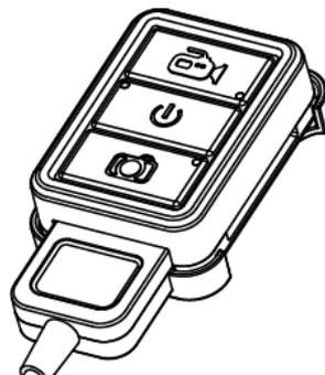
**Charge the Remote Controller:** Place the remote controller to the offered base charger, another USB side to DC 5V, red indicator will turn on beside the POWER button, and will power off after full charged.
