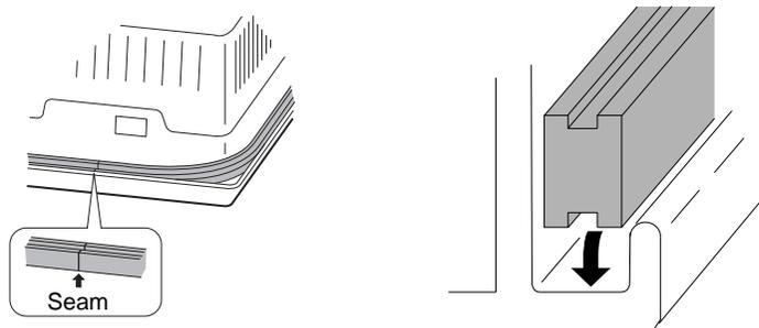
**MEMO** Make sure the gasket is not inserted with its seam (bonded part of the gasket) in any of the corners. If too much force is concentrated on the seam, it may tear.
