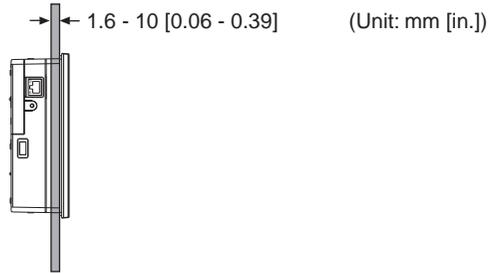
**MEMO** To ensure a sufficient level of water-resistance, make sure the panel is not warped, damaged, or uneven. Attaching reinforcement strips also increases the effectiveness of the PS-G unit’s installation gasket.
