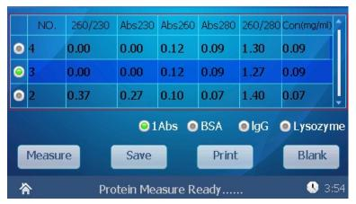
5.4.7 When user want to skim measurement data, press "Tab" to make table in a red frame, as above. Skim tables by press up and down direction key, also can Scroll through the table using the slider bar on the right of the window. Sample type indicated on the table is the one chosen.
