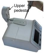
Lower the sampling arm, the sample column is automatically drawn between the upper and lower measurement pedestals.
