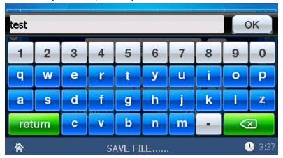
◆ After typing in a file name by keyboard or mouse, click by keyboard or mouse, press "Enter" on keyboard to finish typing. Press "Enter" again or click "OK" to save file. See below, (Notes: When type characters by keyboard, must make sure the previous one is black). Or press "Esc", (Or click "return") to quit.
