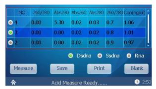
5.3.7 When user want to skim measurement data, press "Tab" to choose table in a red frame, as above. Skim tables by press up and down direction key, also can Scroll through the table using the slider bar on the right of the window. Sample type indicated on the table is the one chosen.
