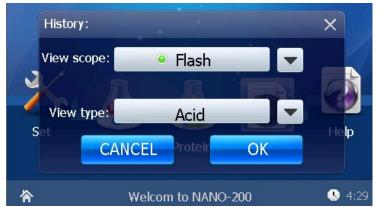
Press "Tab" to make "View scope" turn red, then, press down direction key to choose file position, also can click by mouse or touch pen. Notes, when spot behind the SD is gray, means SD card has not been active or without SD card. This moment, user has to choose "FLASH" as below:
