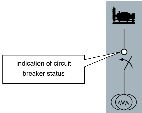
**Genset Indicators :** When ATS transfers load from Mains to the Genset, the LED turns ON if connector 26 detects signal from ATS switch.
