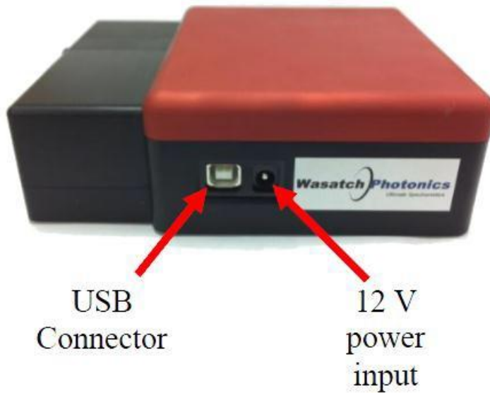
Figure 2 Side view of Stroker 785L with USB port on left and 12V power input on right.
