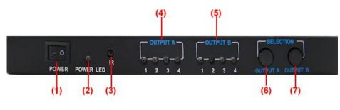
(1). Power Switch (2). Power LED (3). IR Receiving Window (4). LED of Selecting Output A (5). LED of Selecting Output B (6).Switch Button of Output A
