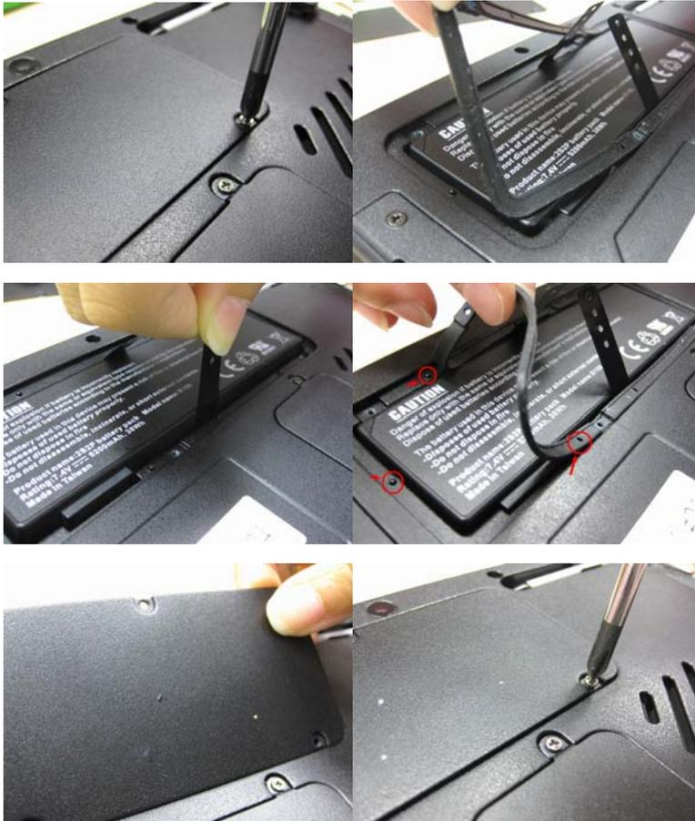
1. Remove the screws on the battery cover at bottom side of your Tablet PC and open the battery cover.
