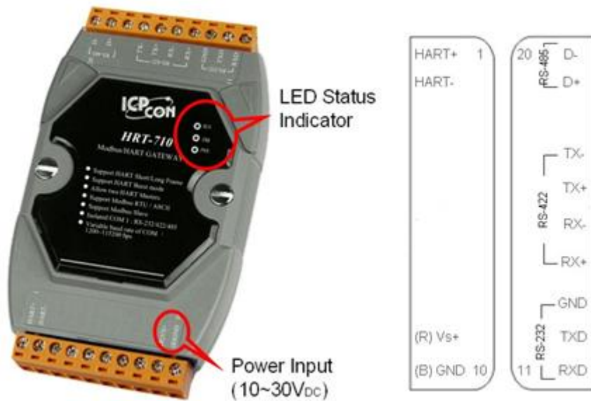
Figure 3: Pin assignment of HRT-710
