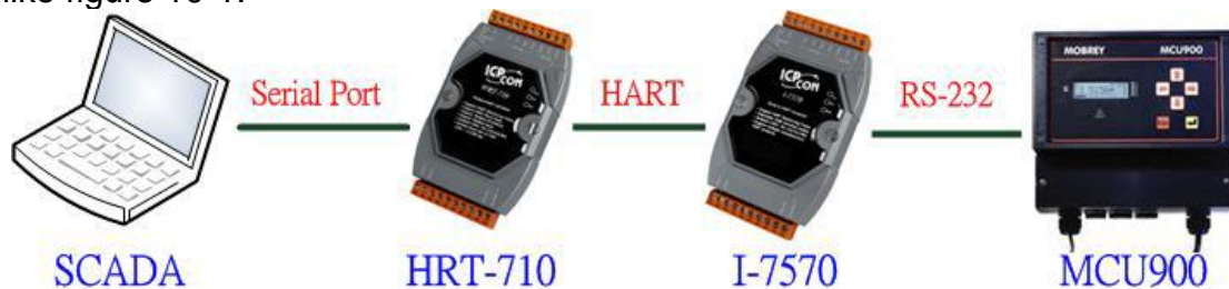
Figure 10-1 The Hardware Wiring for MCU900
