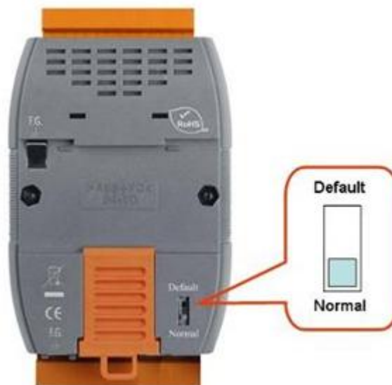
Figure 12: DIP Switch of the HRT-710
