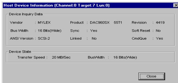
**Figure 5-12. Host Device Information: RAID Controller**
