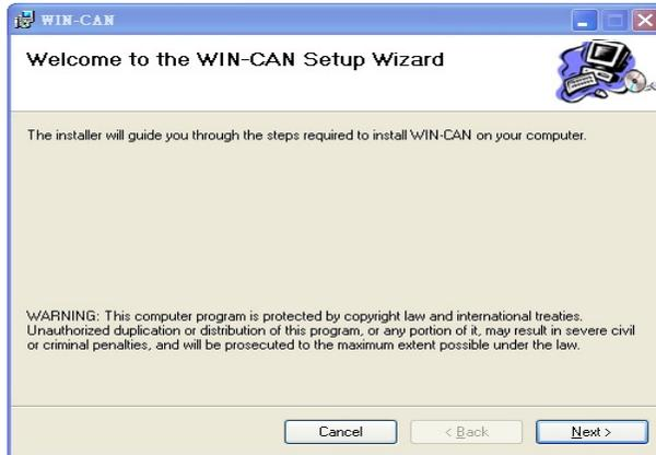
**Step 2:** Click on "Next" to install the USB CAN bus' driver.
