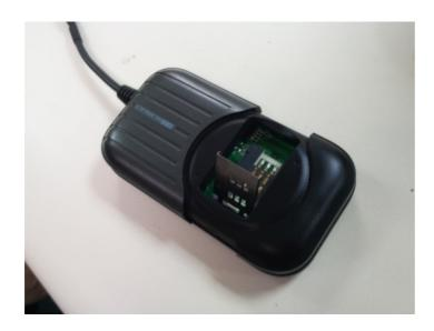
Put the SIM card into the holder, and turn the foil right and fasten it in place.
