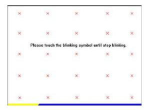
Touch the blinking symbol on panel until beep or stop blinking. After the calibration, the new record will overwrite the old one.
