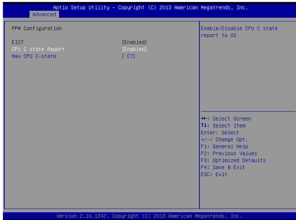
**Figure 3.10 PPM Configuration**
