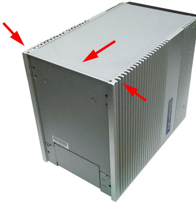
Figure 2.18 Unscrew 2 screws and remove the top cover
