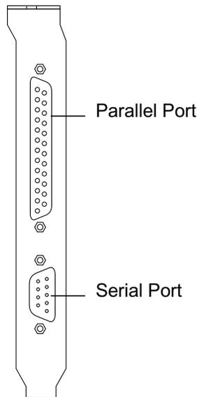
**FIGURE 10-3** SunPCi III Serial/Parallel Port Backplate
