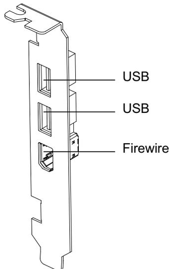
**FIGURE 10-2** SunPCi III USB/Firewire Backplate
