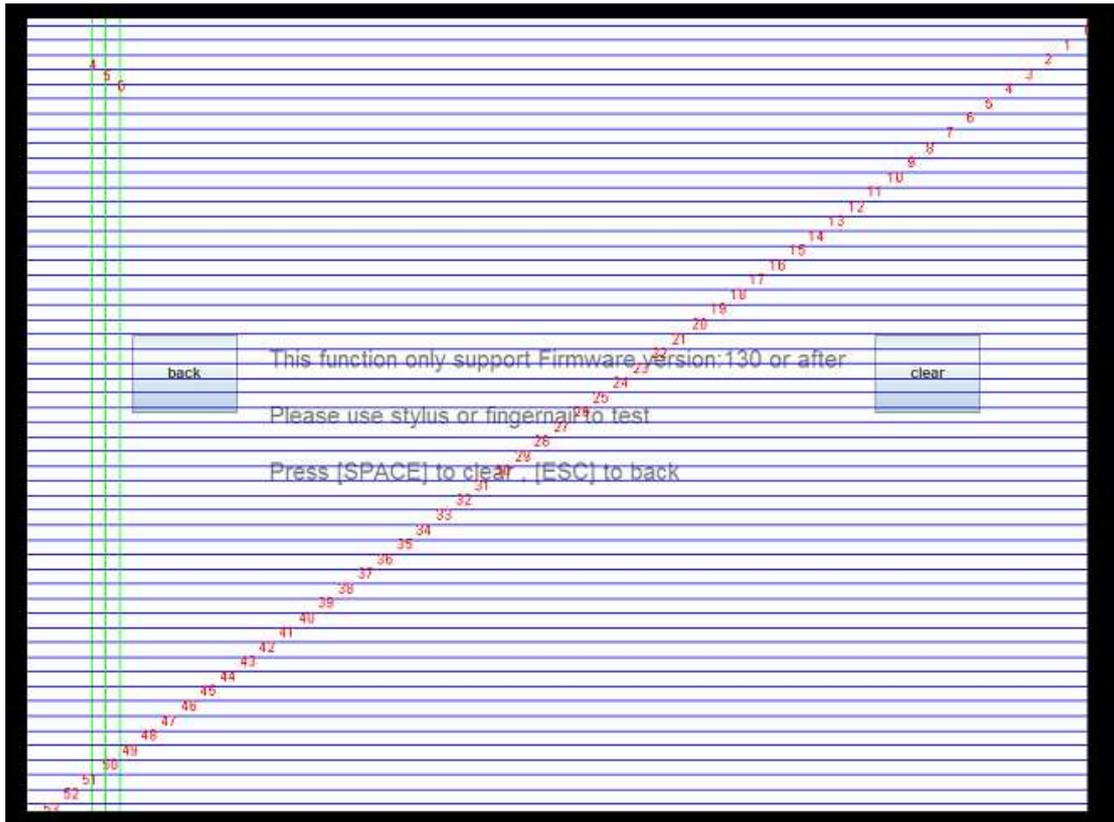
Test Column: from left to right or from right to left to press touch panel, it will draw green line and number, if any number of 0 to NOCOL doesn't appear, It means this number of column maybe open short.
