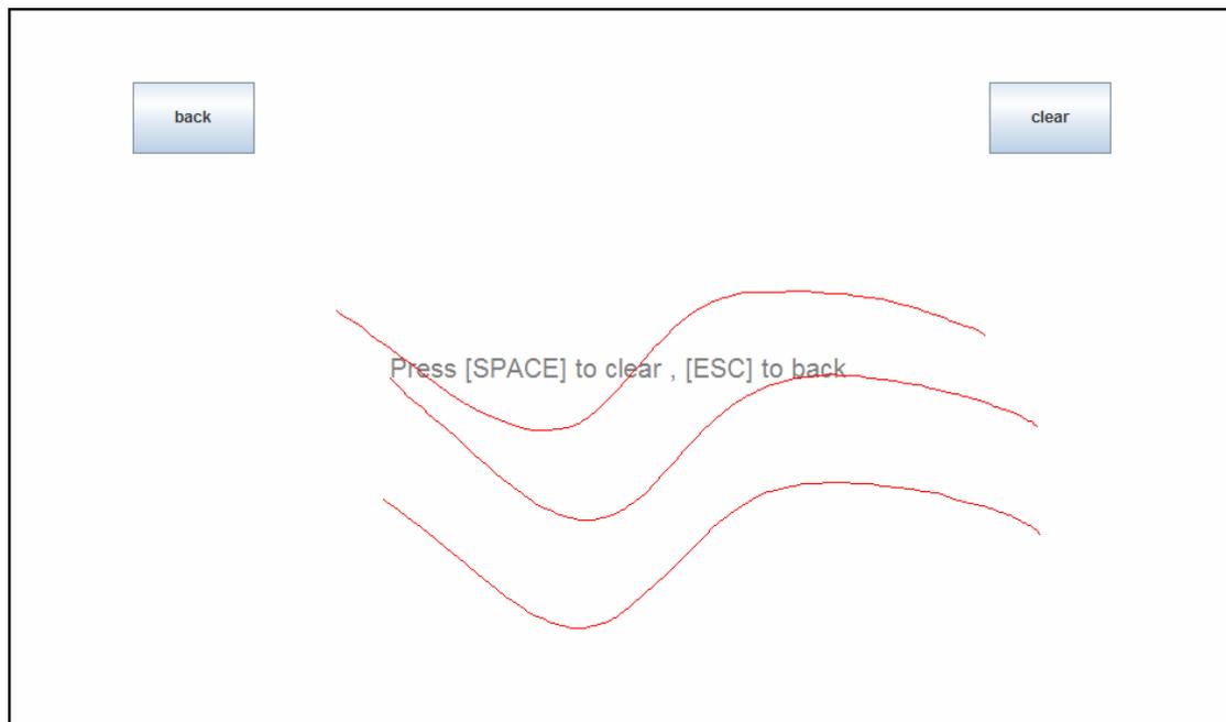
Boundary Test can check touch panel ITO (column and row) are all ok (didn't have open or short condition), or there has some broken ITO line (open) or short point.
