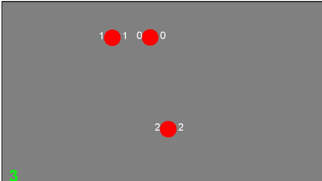
Location Test can check the input point on touch panel is the same as system display point.
