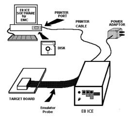
Figure 1.1 ICE System Configuration
