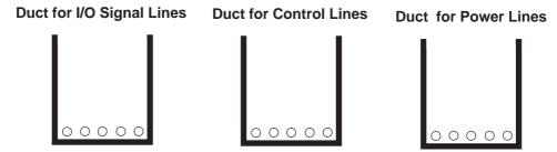
If different wires must be placed in the same duct, separate them with an earthed/grounded divider.
