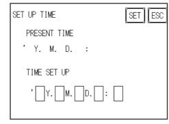
The LT unit's internal clock has a slight error. At normal operating temperatures and conditions, with the LT operating from its lithium battery, the degree of error is ±65 seconds per month. Variations in operating conditions and battery life can cause this error to vary from -380 to +90 seconds per month. For systems where this degree of error will be a problem, the user should monitor this error and make adjustments as necessary.
