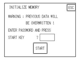
To initialize the LT unit's internal memory, enter the default password, "1101," or the password entered in the SYSTEM SET UP screen.
