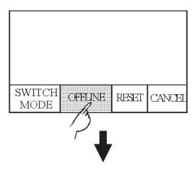
Entering OFFLINE mode will reset the LT unit's I/O. After confirming that this will not cause any problems, touch YES.
