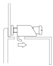
5. Use a Phillips screwdriver to tighten each fastener screw and secure the LT in place.
