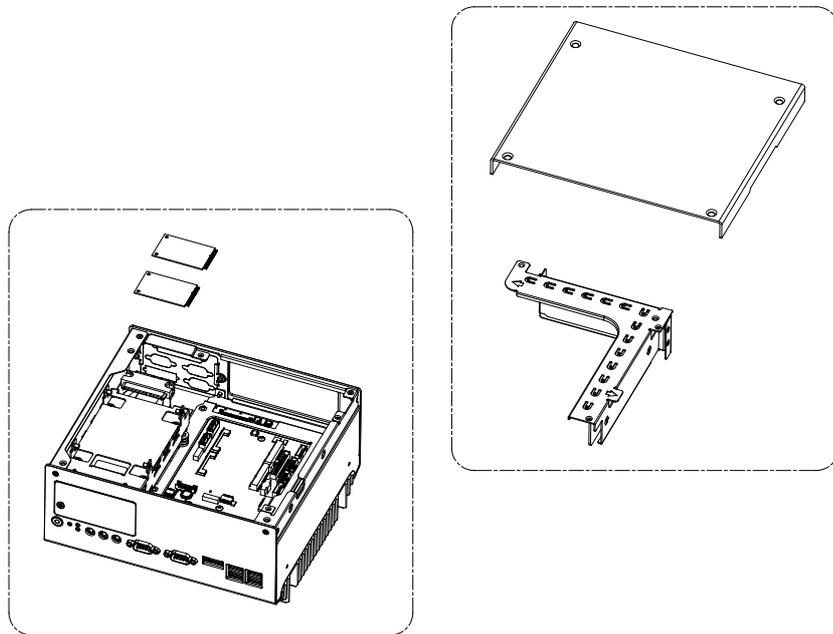
Figure 2.23 Mini PCI Card Installation
