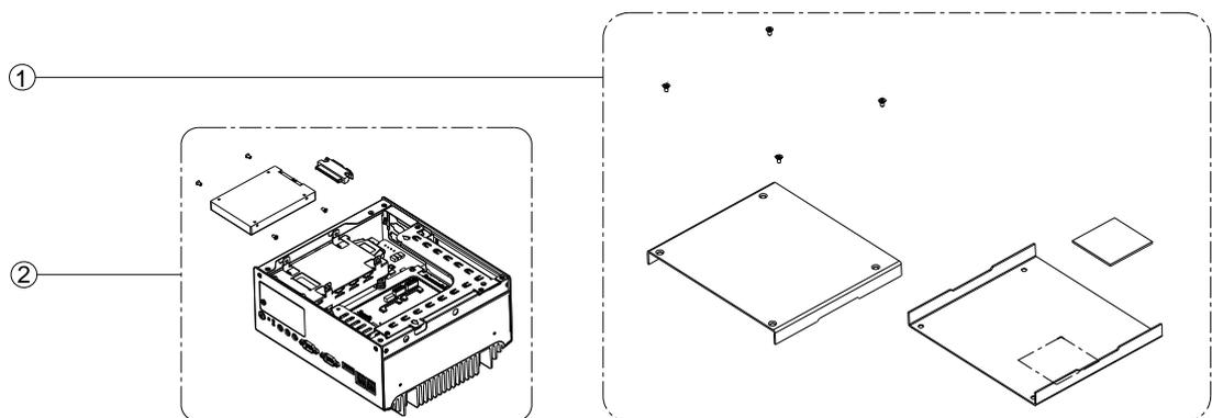
Figure 2.20 Internal Fixed HDD Installation
