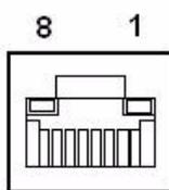
Figure 2.13 Ethernet connector
