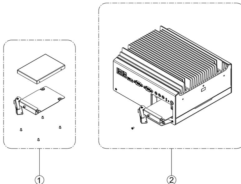
Figure 2.21 Removable 2.5" Storage Device Installation
