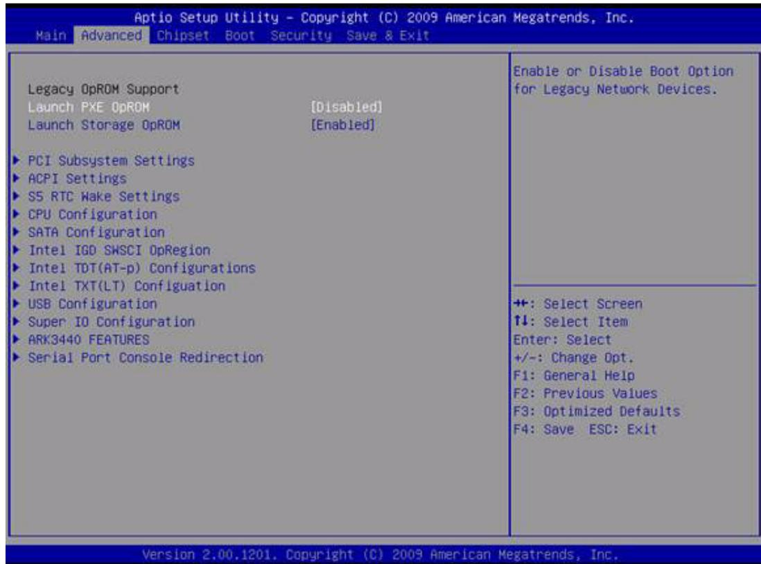
Figure 3.2 The Advanced BIOS setup screen
