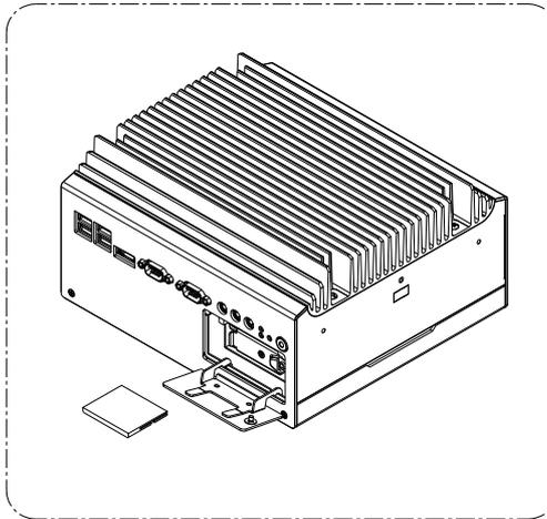
Figure 2.19 CF Card Installation
