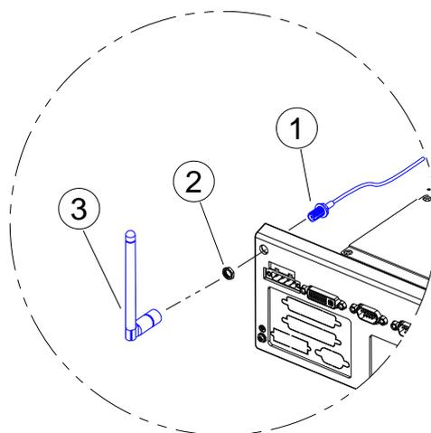
Figure 2.24 Antenna Installation
