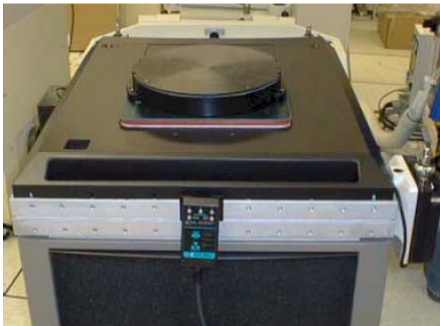
Probe Tower Installed on PIB
