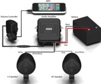
Figure 5. Wiring diagram of Moto-820 / Moto-825 / Moto-830.
