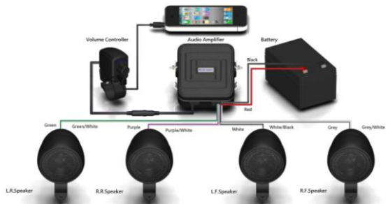
Figure 5. Wiring diagram of Moto-820 / Moto-825 / Moto-830.
