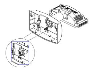
5. Cover the Stand Plate back and fasten the screws.
