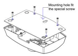
6. You may use the enclosed mounting screws (one Special screw and two Wood screws) to fix the Display on the wooden table surface.
