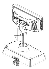
Connect the cable from the Display to the XH connector inside the Stand until you feel it clicked. Also connect the enclosed USB cable to the "USB" connector.
