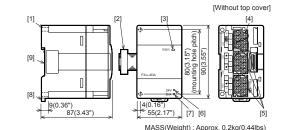
[1] Direct mounting hole:2 holes of  $\phi4.5$  (0.18") (mounting screw: M4 screw) [2] Extension cable
