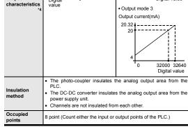
\*1 Change the offset and gain values to change the output characteristics. However, the resolution doesn't change even when the offset and gain values
