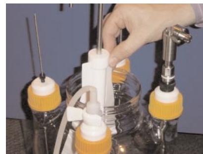
Figure 19. Straighten paddle blades after insertion
