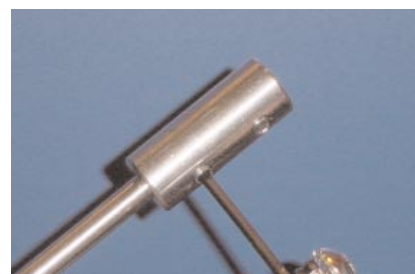
Figure 9. Tighten lower set screw (Step 5).
