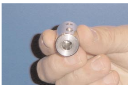
Figure 6. Coupling collar – larger opening for paddle shaft
