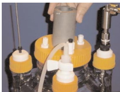
Figure 20. Place cap on flask and tighten
