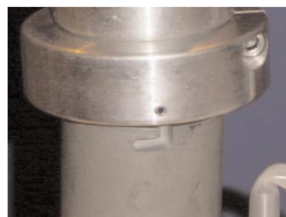
Figure 24. Correct orientation of motor on Drive Shaft
