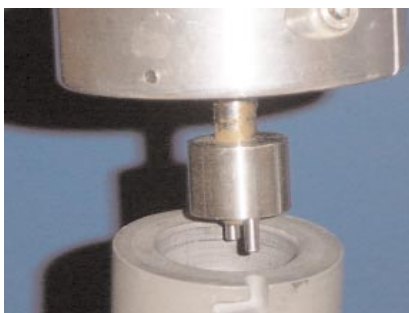
Figure 23. Coupling of motor and Direct Drive Shaft
