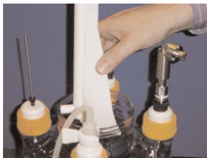
Figure 18. Insert the assembled paddle into flask (bend paddle if necessary)
