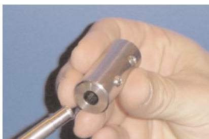
Figure 8. Slide larger opening on coupling collar over paddle shaft (Step 4).
