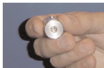
Figure 7. Coupling collar – smaller opening for drive shaft
