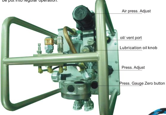
3.3 Adjusting The Pressure Regulating Valve
