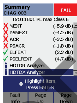
Figure 8: Access HDTDX and HDTDR data by selecting the parameters. They are shown at the end of the list of test parameters. They are not test parameters as defined by the standards. The 'i' symbol before their names indicates "for information only."
