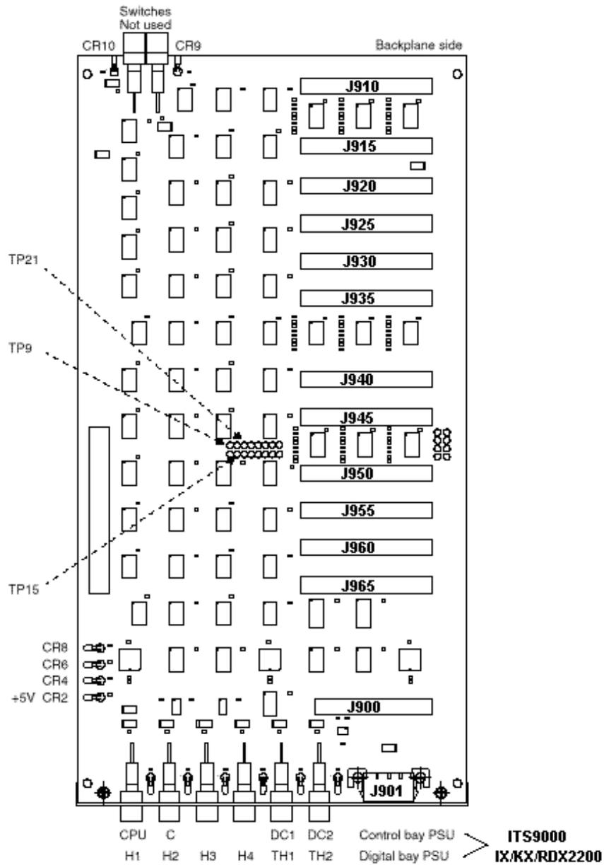
Figure 3: PSU Board Layout, Part Number 794000702
