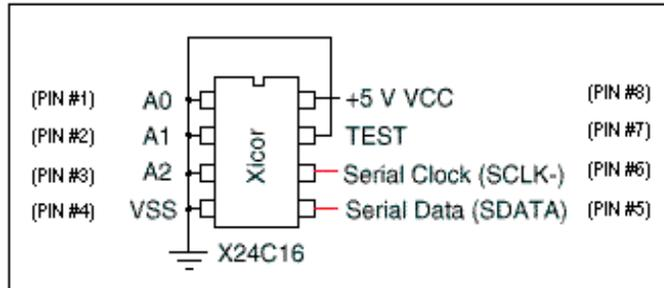
Figure 6: Schematic of Loadboard EEPROM Device
