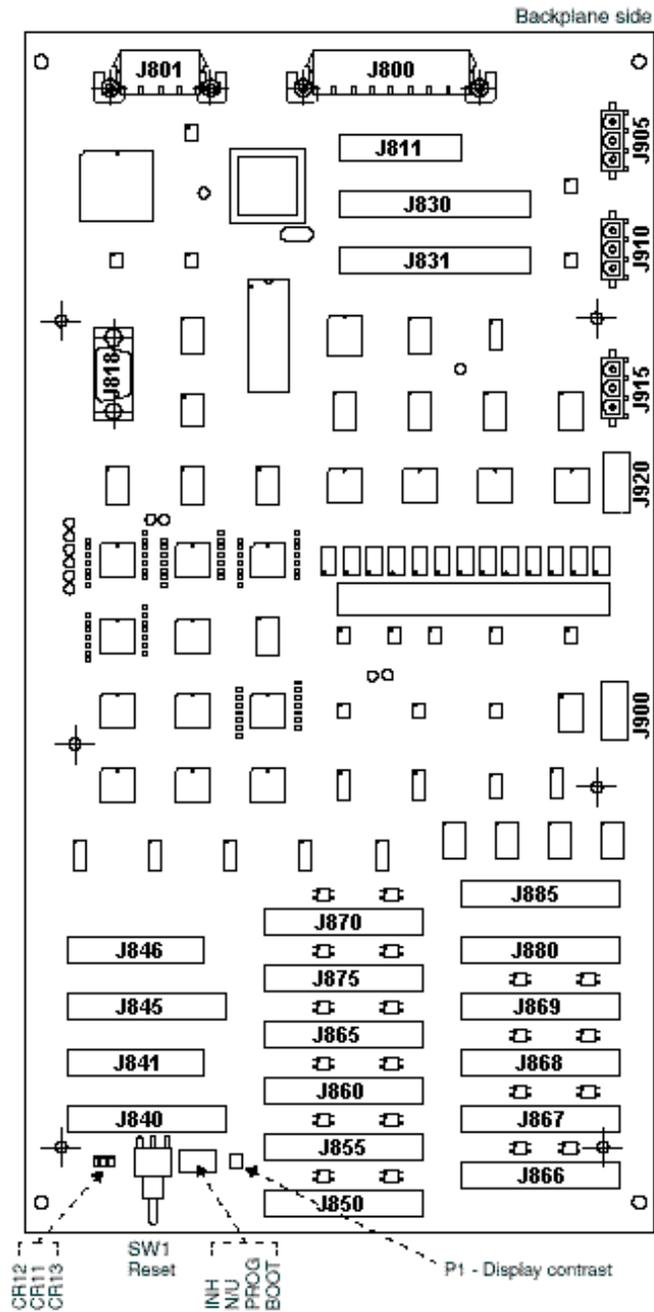
Figure 2: Alarm Board Layout, Part Number 794000701
