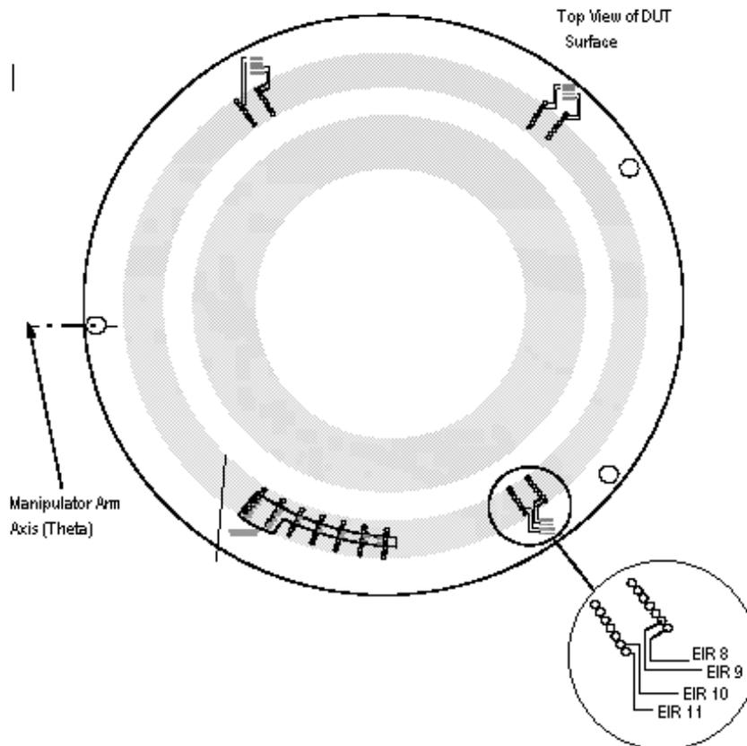
Figure 8: EIR Bit Pogo Pin Location
