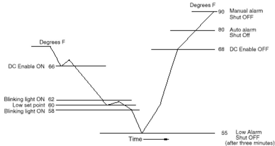
Figure 1: Heat Exchanger Normal Operating Set Point Operational Sequence
