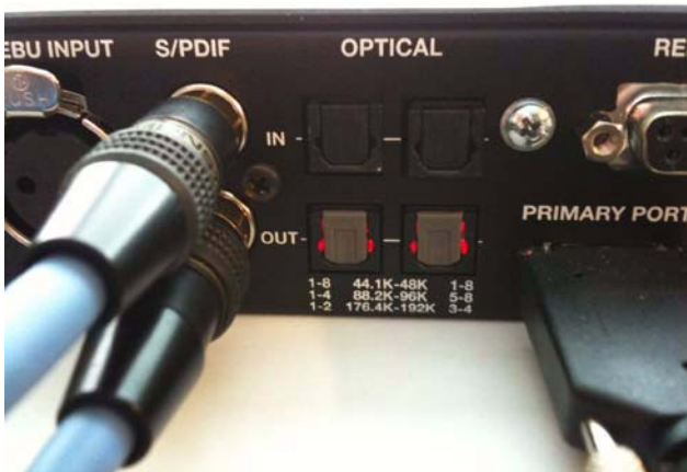
Figure 10. Coaxial (S/PDIF) loop back connections
