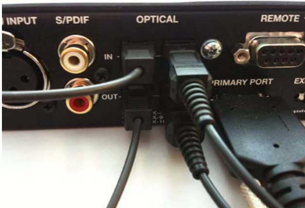
Figure 7. Optical loop back connections
