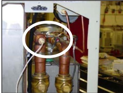
3. Unplug the sensor from below the control box.
