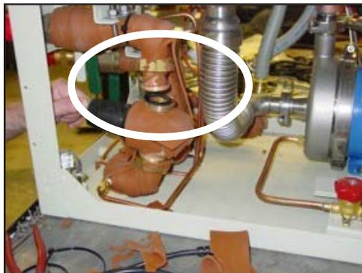
6. When installing new regulator and washers ensure the arrow on the side of the regulator points down.
