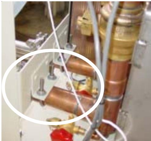
7. Undo the sanitary fitting at the tank.
