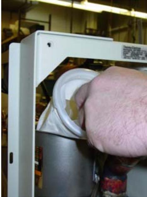
7. Install a new bag. **Ensure that the paper tag is removed from the bag.**
