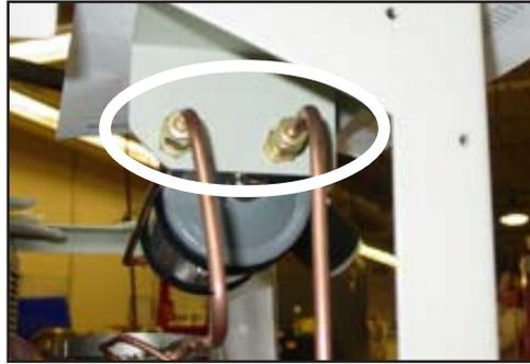
6. Undo the u-bolts securing the line to the unit.
