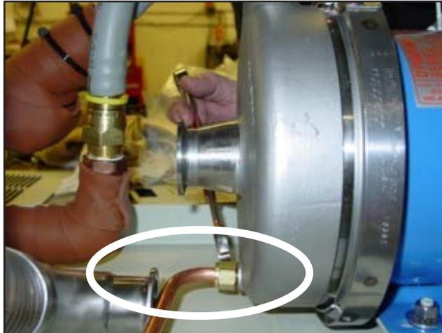
5. Using a 7/16" wrench, remove the 6 bolts securing the pump plate to the unit.
