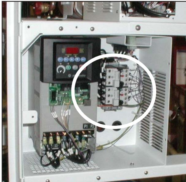
3. When installing, torque all screws to 24 - 28"-lbs.
