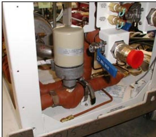
4. Unplug the 6-pin connector and disconnect the ground wire.
