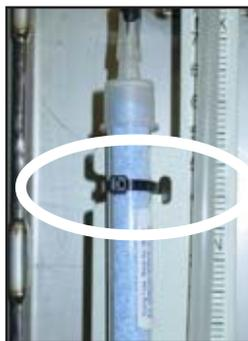
3. Reverse the procedure to install a new dryer tube.
