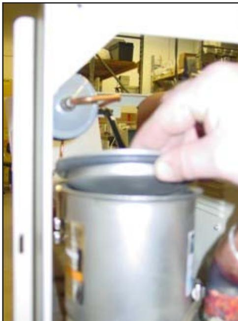
10. To reinstall a new bag push down on the lid and gasket when tightening the black knob. Hand tighten until the gap matches the other two gaps.
