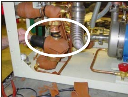
4. Undo the u-bolts securing the plumbing to the bottom of the unit's midpan.
