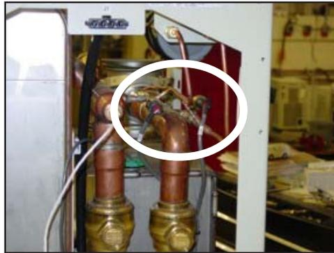
2. Use the 5/8" wrench to disconnect the transducer(s).
