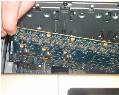
Figure 3. Sliding the front of the card into PCIe card support
