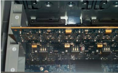
Figure 4. PCIe card installed
