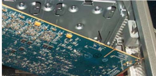
Figure 2. Holding the card above the slot at an angle
