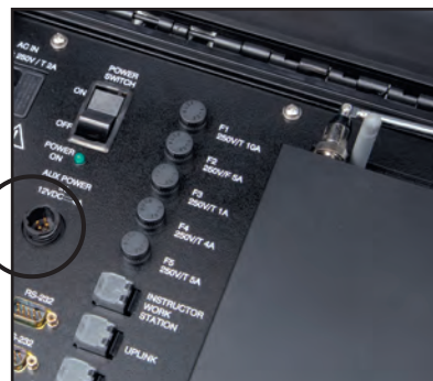
The PCU's Auxiliary Power Port
