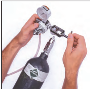
Attaching the CO 2 Regulator
