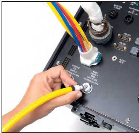
Connecting Air or CO 2 to the PCU
