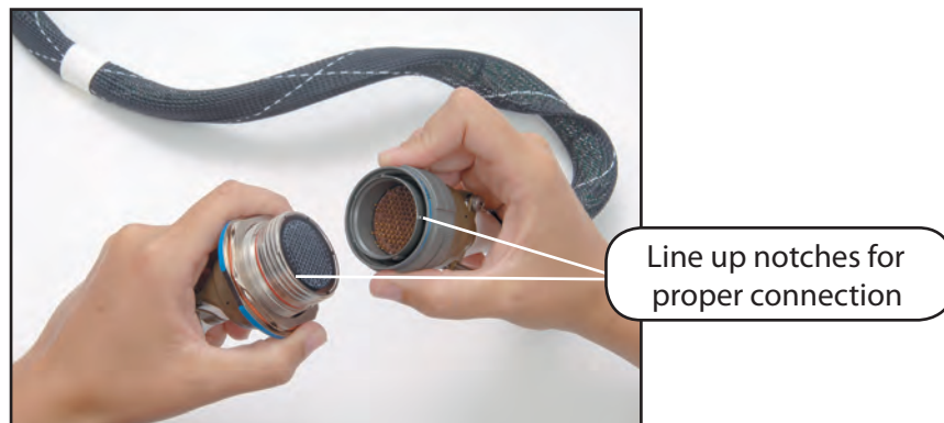
Electrical Connection to Umbilical
