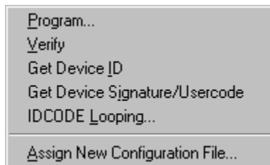
Figure 4-10 Available Boundary-Scan Operations for a Virtex device
